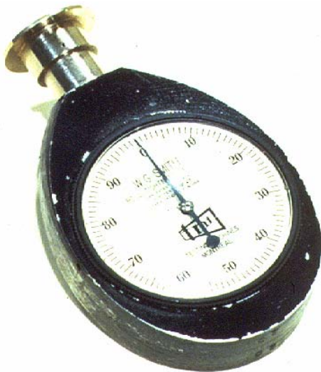
Smith Needle AccuWind Roll Density Curve Hardness Devices for Measuring Roll Hardness From Core to Full Roll
