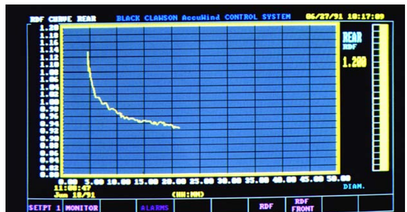
Smith Needle AccuWind Roll Density Curve Hardness Devices for Measuring Roll Hardness From Core to Full Roll
