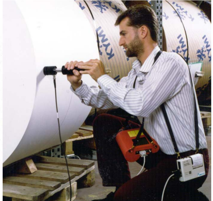
Rhometer PAROtester Hardness Devices for Measuring Roll Hardness Across Roll
